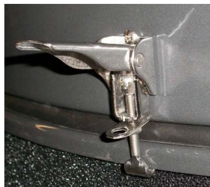
Detail showing tension screw and locknut. This has been adjusted and locked in the factory for correct tension and an airtight seal. Do not tamper with the locknut. If setting is changed for any reason, check for tight fit before completing the installation.
